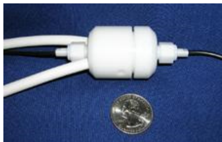
Figure 29: Prototype of a optical (high) voltage sensor developed by PPI.
